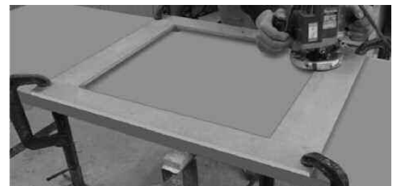
Fig. 4 Hob/Sink template clamped in position
